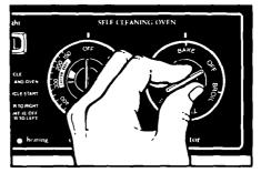
2. Set the Oven Selector on BAKE. The Oven ON Indicator Light will come on.
