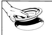
2. Line up openings in the reflector bowl with the surface unit receptacle and the element hold down clip.
