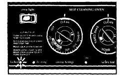
5. The Oven LOCKED Indicator Light comes on when the oven temperature exceeds normal baking temperatures. The Lock Lever must not be moved and the door can't be opened when the Oven LOCKED Indicator Light is on.
